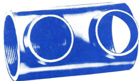
Type HM2 for welded frame 1.370 x 24 TPI BSC Thread 68mm wide. Chainstay pipes 22.2mm I/D 38mm between centres. V. Pattern (for straight stays)
